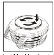
fig. 11 - fit side plate
